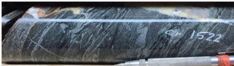
Qtz-Mt-Py vein (left) in chlorite-sericite altered ultramafic tuff (16.2m).
