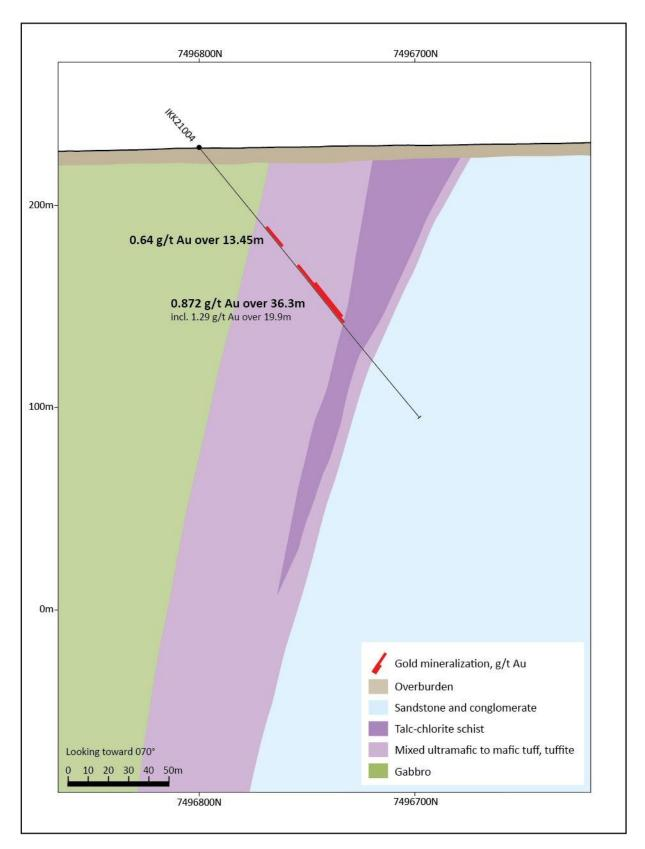
Figure 3: Cross section hole IKK21004.
