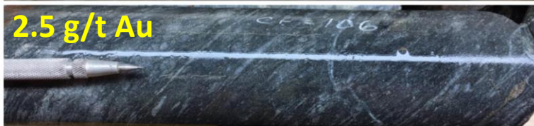
Sheared Mt-Sil-FeCarb-Chl tuffite hosting 0.5-1% fine-grained Py (35.4 and 36.6m).
