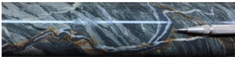
Discordant Qtz-Mt vein in ultramafic tuff (27.5m).
