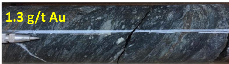
Discordant Qtz-Mt vein in ultramafic tuff (27.5m).
