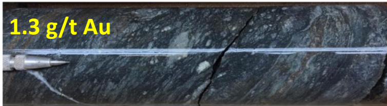
Discordant Qtz-Mt vein in ultramafic tuff (27.5m).
