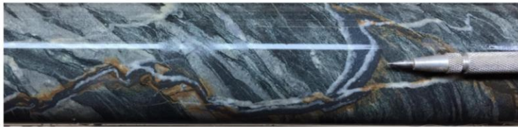
Discordant Qtz-Mt vein in ultramafic tuff (27.5m).
