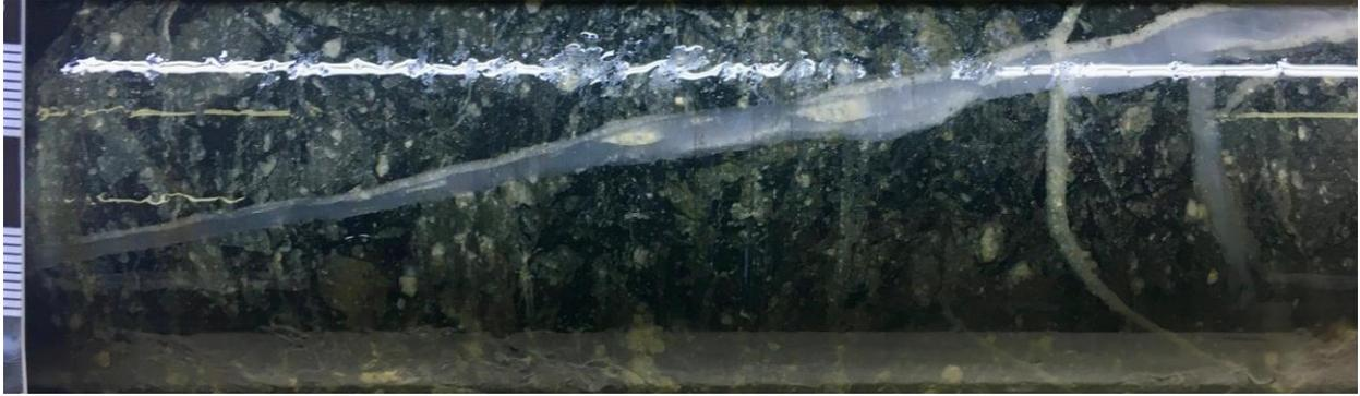
**Figure 4: Drill hole KUE22027. Brecciated Fe-dolomite and Qtz veins in high strain silica-tourmaline breccia cut by Qtz and Fe-dolomite veinlets at 173.35 m within interval of 1.56 g/t Au over 24.8 m from 159.0 m.**
