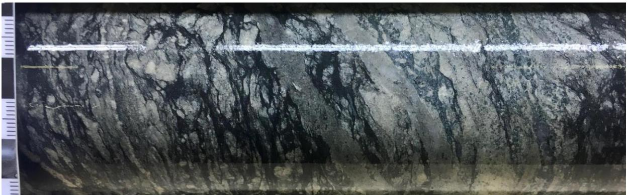
**Figure 5: Drill hole KUE22027. Biotite-chlorite altered sheared ultramafic tuff with abundant polyphase Fe-dolomite veins representing proximal halo around mineralized lens at 179.5 m within interval of 1.56 g/t Au over 24.8 m from 159.0 m.**
