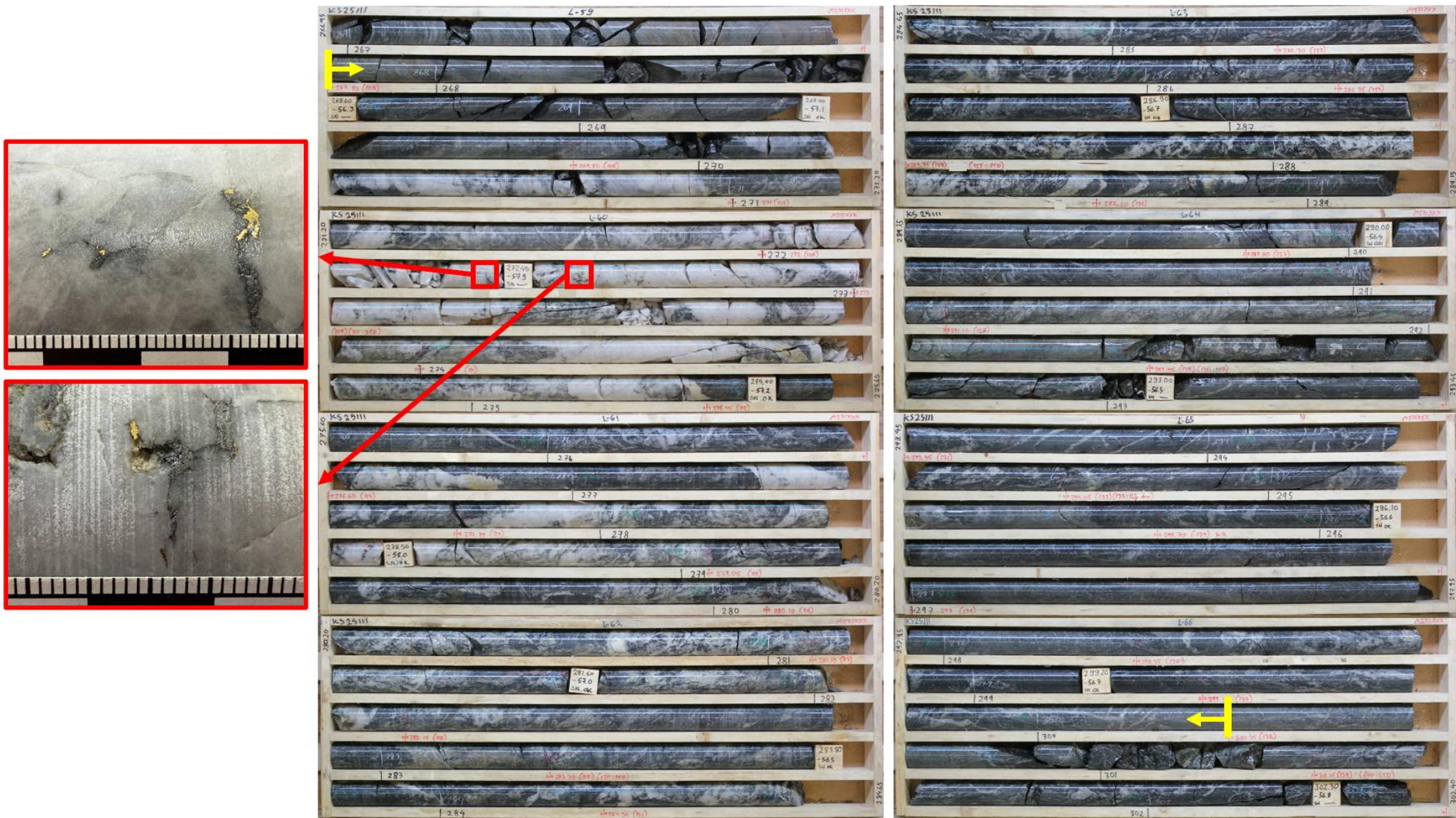
Figure 6: Gold mineralization, 4.42 g/t Au over 32.55 m from 267.80, in drill hole KS25111, Vanha prospect, Kaarelselkä area, Risti property
