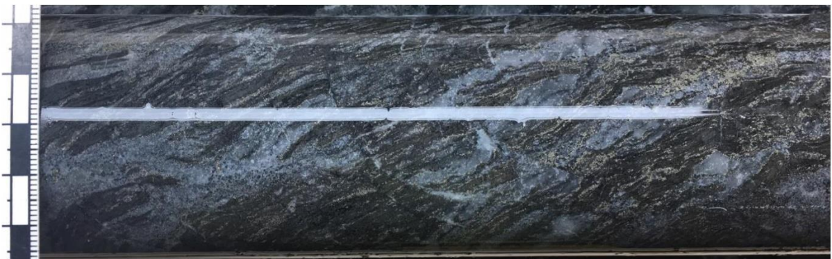
Chl-Bt-Mt-altered tuffite (TFT) hosting 7-15% of fine-grained PY (132-133m and 134m).
